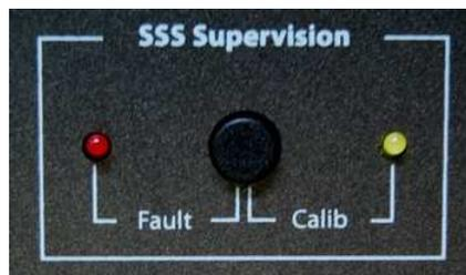
*Figure 2 : User interface of the SSS option on the UT26 processor front panel.*
