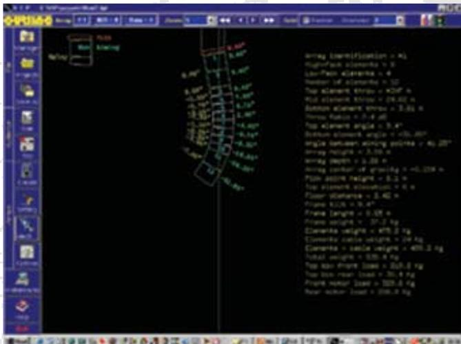
An accurate prediction of the angle between the elements, even if they're a mixture of Hi-Packs and Low-Packs, greatly facilitates "aiming" at the audience. Riggers are thus provided with all the geometric and mechanical data necessary for carrying out their work perfectly, without worrying about committing any serious mistakes. A diagram is created for each array, with all the parameters for flying according to the limits set by international safety norms for suspended loads.
