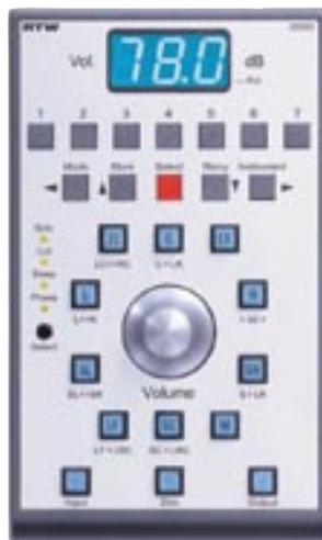
illuminated buttons duplicate those at the bottom of the screen. A small inset button and indicator LEDs determine the function of buttons set around the volume knob to Solo, Cut, Swap or Phase. Solo and Cut are non-additive unless multiple keys are depressed together. At the bottom, three buttons change Input and Output selections with the Dim key in the middle. There is no separate Master Cut, although the Dim key can be programmed to be Cut.
